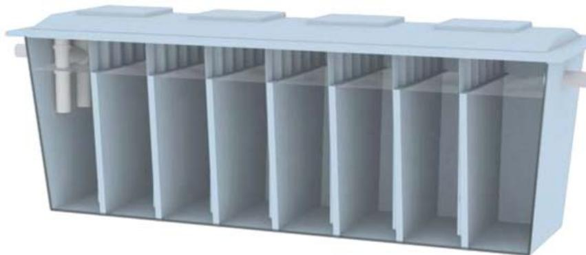
**Figure 4:** A prefabricated anaerobic baffled reactor, aimed to treat about 10 day (drawing: courtesy of BORDA<sup>1</sup>)
