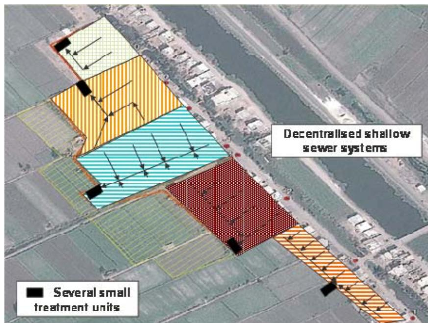
**Figures 1&2:** Comparison of a fully centralised scenario with conventional sewer system (above) and a decentralised scenario, featuring several shallow sewer systems and modular treatment units. Case study of Iz. Islah, Beheira (drawing: Jörg Haucke)
