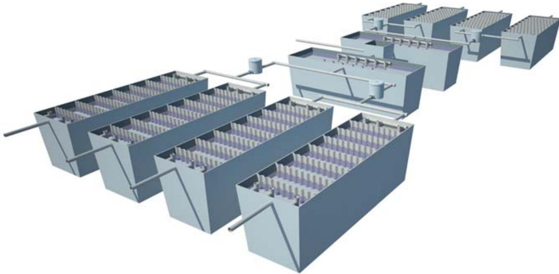
**Figure 3:** Modular prefabricated treatment units, consisting, in that case, of 2 prefabricated settlers and 8 prefabricated anaerobic baffled reactors (ABR), treating about 80 m<sup>3</sup>/day (drawing: courtesy of BORDA<sup>1</sup>)
